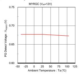
(15) PG Output Voltage vs. Ambient Temperature
