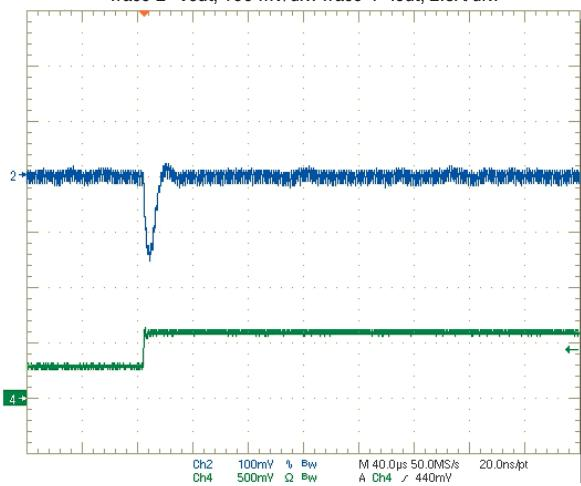
Step Load Transient Response (Vin=12V, Vout=1.2V, Cload=0, Iout=3A to 1.5A)
