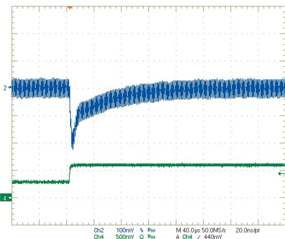
Step Load Transient Response (Vin=12V, Vout=5.0V, Cload=0, Iout=3A to 1.5A)
