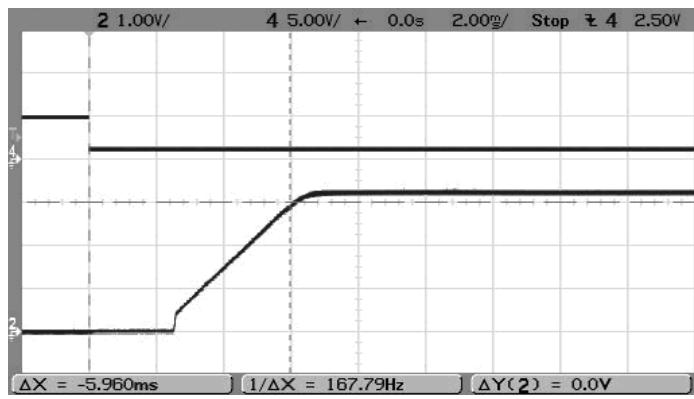
Step Load Transient Response (Vin=12V, Vout=3.3V, Cload=0, Iout=1.5A to 3A)
