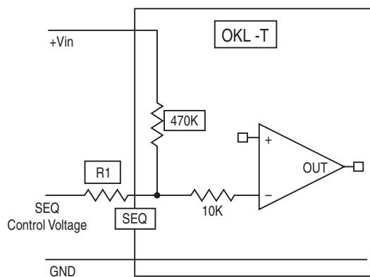
Figure 7. Sequencing Signal Interface of Module
