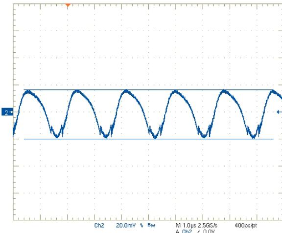
Step Load Transient Response (Vin=12V, Vout=2.5V, Cload=0, Iout=1.5A to 3A)
