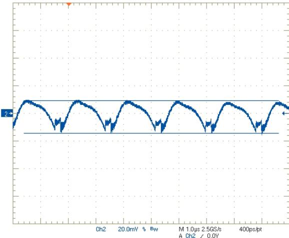
Step Load Transient Response (Vin=12V, Vout=1.2V, Cload=0, Iout=1.5A to 3A)
