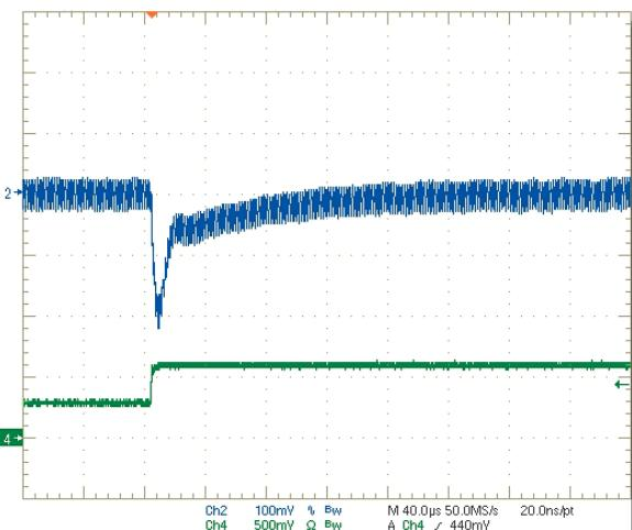
Output Ripple and Noise (Vin=12V, Vout=3.3V, Iout=3A, Cload=0, ScopeBW=20MHz)
