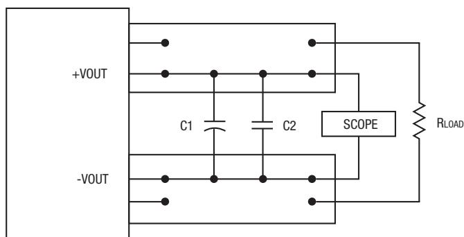
Figure 5. Measuring Output Ripple and Noise (PARD)
