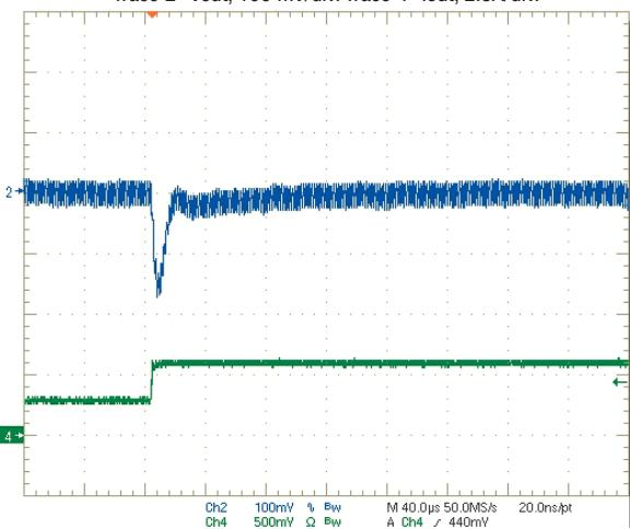
Step Load Transient Response (Vin=12V, Vout=2.5V, Cload=0, Iout=3A to 1.5A)
