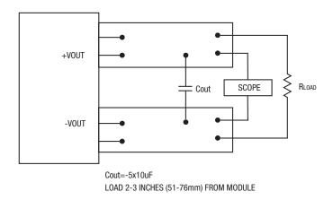
Figure 5: Measuring Output Ripple and Noise (PARD)
