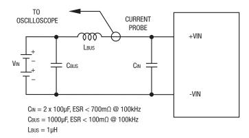
Figure 4: Measuring Input Ripple Current
