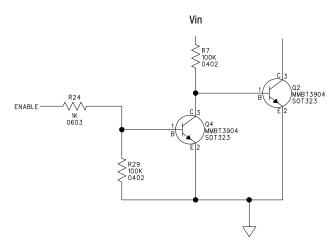
Figure 6. On/Off Control Circuit
