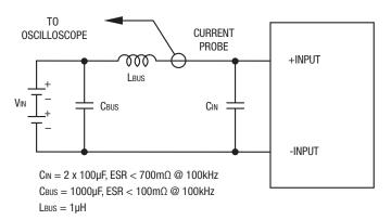
Figure 2: Measuring Input Ripple Current
