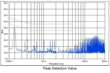
Graph 2. Conducted emissions performance, Negative Line, CISPR 22, Class B, 48 Vin, full load
