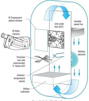
Figure 11. Vertical Wind Tunnel
