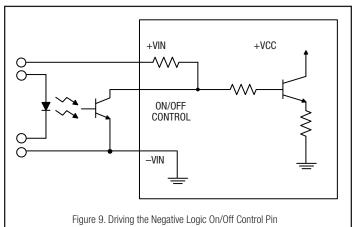
Dynamic control of the On/Off function should be able to sink appropriate signal current when brought low and withstand appropriate voltage when brought high. Be aware too that there is a finite time in milliseconds (see Specifications) between the time of On/Off Control activation and stable, regulated output. This time will vary slightly with output load type and current and input conditions.
