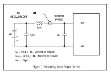
multiple external capacitors. Be sure to calculate component temperature rise from reflected AC current dissipated inside capacitor ESR. Our Application Engineers can recommend potential solutions.
