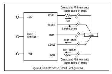
Output overvoltage protection is monitored at the output voltage pin, not the Sense pin. Therefore excessive voltage differences between Vout and Sense together with trim adjustment of the output can cause the overvoltage protection circuit to activate and shut down the output.
