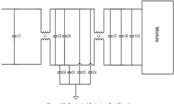
Figure 10. Conducted Emissions Test Circuit
