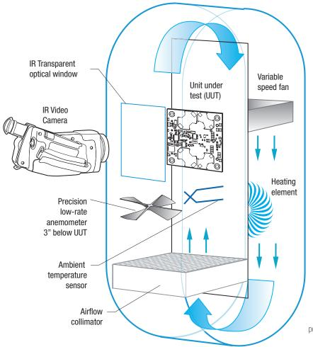
Figure 14. Vertical Wind Tunnel
