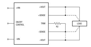
cause the overvoltage protection circuitry to activate (see Performance Specifications for overvoltage limits). Power derating is based on maximum output current and voltage at the converter's output pins. Use of trim and sense functions can cause output voltages to increase, thereby increasing output power beyond the converter's specified rating or cause output voltages to climb into the output overvoltage region. Therefore:
