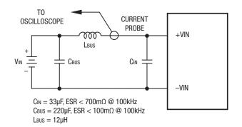
Figure 2. Measuring Input Ripple Current
