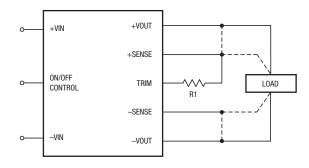
between Vour and Sense, in conjunction with trim adjustment of the output voltage, can
