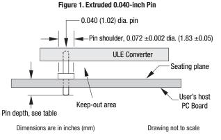
The "integral" pin shoulder is formed as part of the extruded pin fabrication and replaces the plastic standoff spacer. The shoulder diameter is 0.072 + -0.002" and forms the mounting plane of the converter. The user should provide sufficient clearance for a 0.040" pin hole but well below the 0.072" shoulder diameter. This mounting plane avoids mechanical stress placed on the converter components. Do not place the components below the converter.
