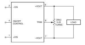
Figure 5. Trim Connections Using A Trimpot
