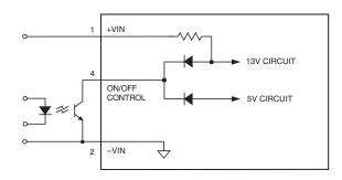
Figure 2. Driving the Positive Logic On/Off Control Pin
