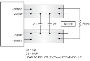
Figure 3. Measuring Output Ripple/Noise (PARD)
