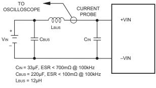
Figure 2. Measuring Input Ripple Current
