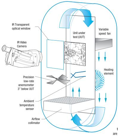
Figure 8. Vertical Wind Tunnel
