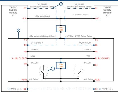
Pin C2 shown here configured for "RAPID\_On" (Cold Redundant bus). For applications requiring an INPUT\_OK signal (default setting), refer to "Status and Control Signals" table for details
