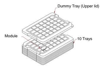
11 trays, desiccant and humidity indicator are packed into a moisture shielding bag. Inner box contains one bag.
