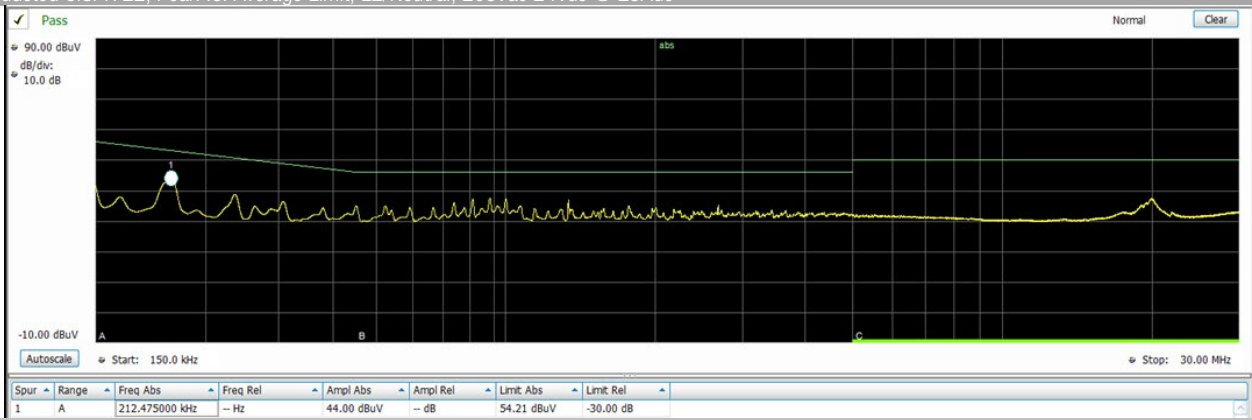
EMI; Conducted CISPR 22; Peak vs. Average Limit; L2/Neutral; 208Vac 24Vdc @ 25Aac
