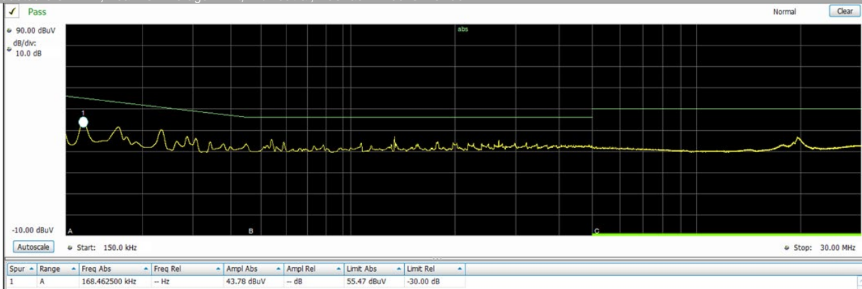
EMI; Conducted CISPR 22; Peak vs. Average Limit; L1; 208Vac 24Vdc @ 25Aac
