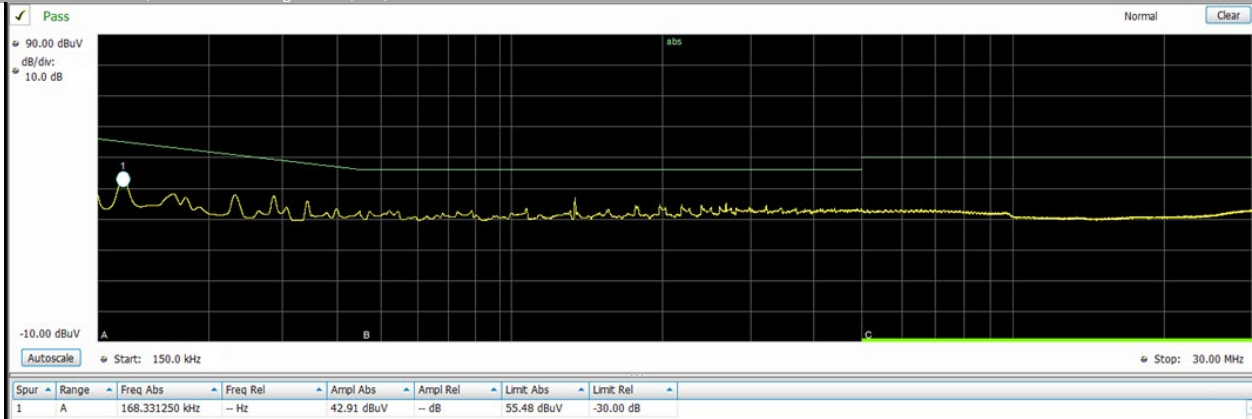
EMI; Conducted CISPR 22; Peak vs. Average Limit; L2/Neutral; 100Vac 24Vdc @ 25Aac
