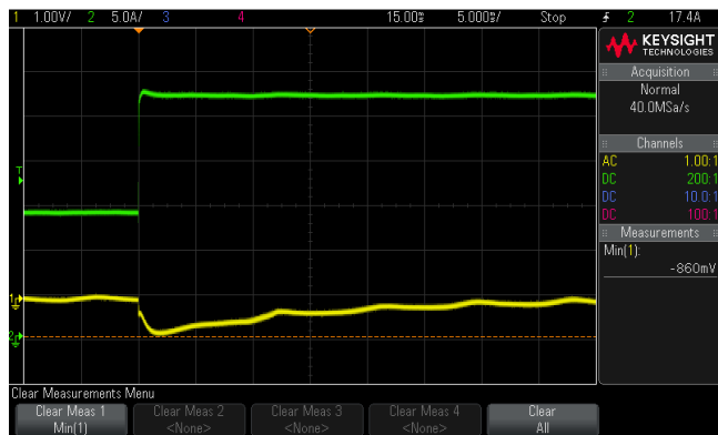
Inrush Current; 264Vac input, Cold Start, 10.5A pk
