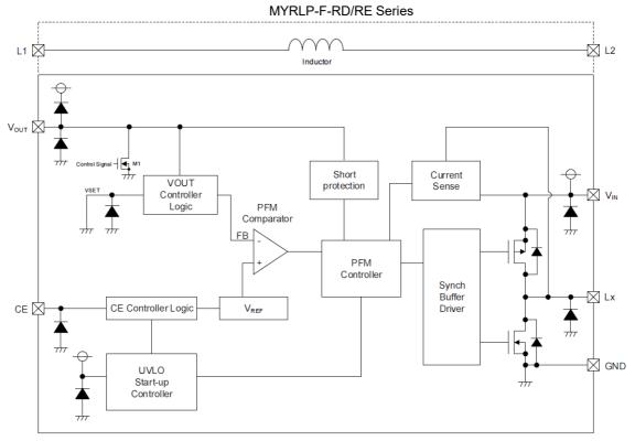
$<sup>^{\</sup>star}$  Diodes inside the circuits are ESD protection diodes and parasitic diodes. MYRLP-F-RE does not have C<sub>L</sub> Discharge function.
