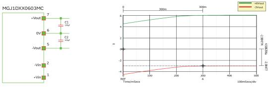
To avoid spurious gate pulses it is recommended that the PWM gate signal is not applied until after the settling time has ended. An alternative method to reduce the settling time is to adjust the values of the additional capacitance so that the CV products are equal. i.e.  $C3 \times 6V = C4 \times 3V$ . So, for instance if a maximum capacitance of 75uF is applied to the +6V output and 150uF is applied to the -3V output the settling time is greatly reduced.
