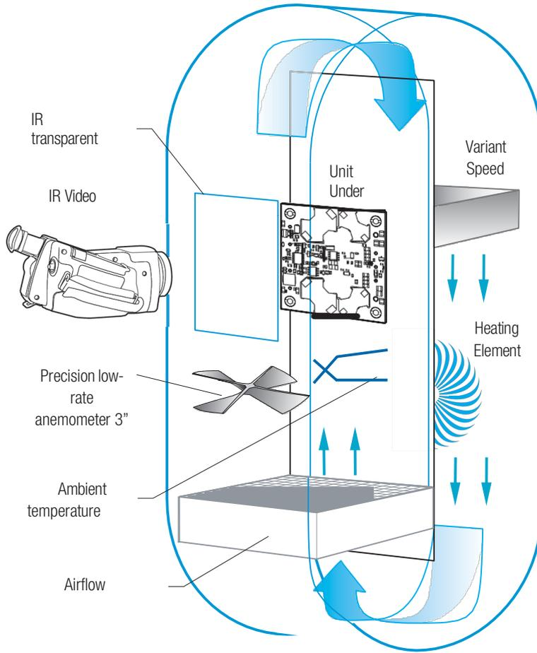
Figure 27. Vertical Wind Tunnel
