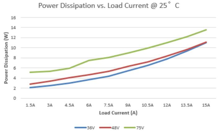
Figure 18. Power Dissipation vs. Load Current @ 25° c
