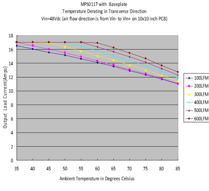
Figure 13. Temperature Derating – Transverse Direction
