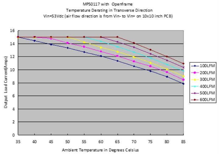
Figure 20. Temperature Derating – Transverse Direction Vin=53Vdc (air flow direction is from Vin- to Vin+ on 10x10 inch PCB)
