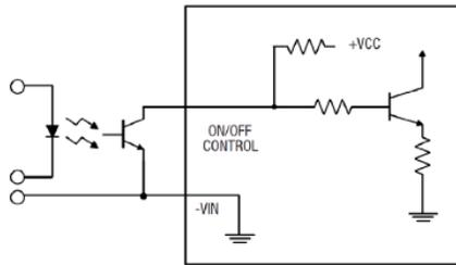
Figure 26. Driving the On/Off Control Pin (suggested circuit)
