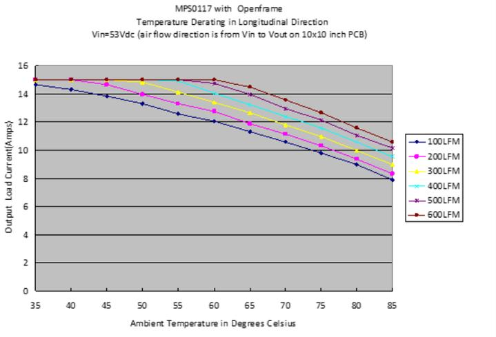
Figure 22. Temperature Derating – Longitudinal Direction Vin=53Vdc (air flow direction is from Vin to Vout on 10x10 inch PCB)
