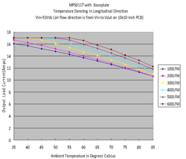
Figure 16. Temperature Derating – Longitudinal Direction
