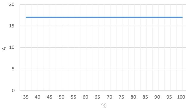
Figure 5. Output Current Derating – Cold Wall
