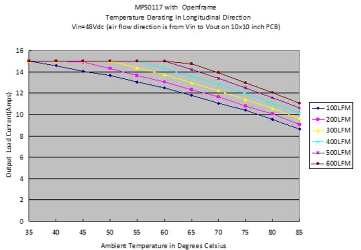
Figure 21. Temperature Derating in Longitudinal Direction Vin=48Vdc (air flow direction is from Vin to Vout on 10x10 inch PCB)
