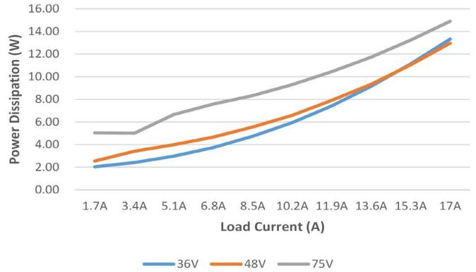
Figure 8. Power Dissipation Vs. Load Current @ 25°C
