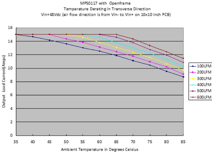
Figure 19. Temperature Derating – Transverse Direction Vin=48Vdc (airflow is from Vin- to Vin+ on 10"x10" PCB)
