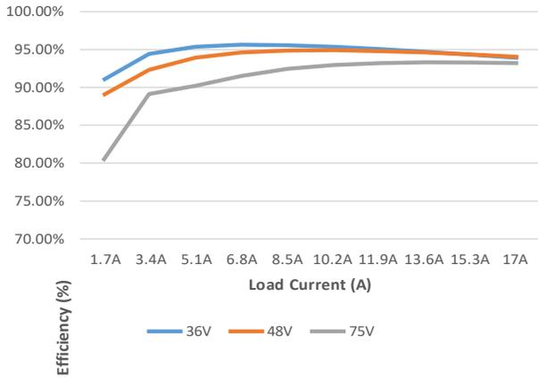
Figure 7. Efficiency Vs. Line Voltage & Load Current @ 25°C
