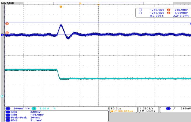
Figure 9. Output Transient Response
