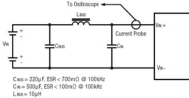
Figure 23. Measuring Input Ripple Current
