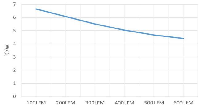
Figure 6. Thermal Resistance – Baseplate
