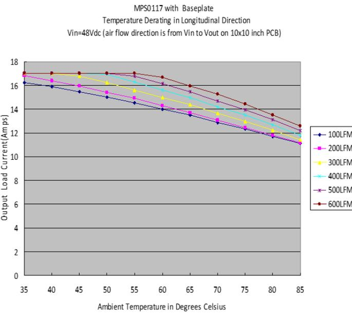
Figure 15. Temperature Derating – Longitudinal Direction
