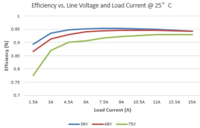
Figure 17. Efficiency vs. Line Voltage and Load Current @ 25° c
