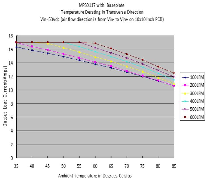
Figure 14. Temperature Derating – Transverse Direction
