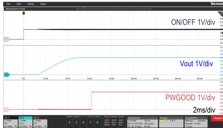
Figure 6. Start-up Waveform ( V_{IN}=12V , V_{OUT}=5.0V , I_{OUT}=10A , C_{OUT}=400\mu F )
