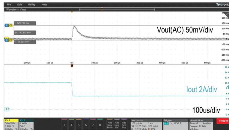
Figure 9. Load Transient Response Waveform ( V_{IN}=12V , V_{OUT}=5.0V , C_{OUT}=400\mu F , I_{OUT}=5 to 10A ( 1.0A/\mu s ))
