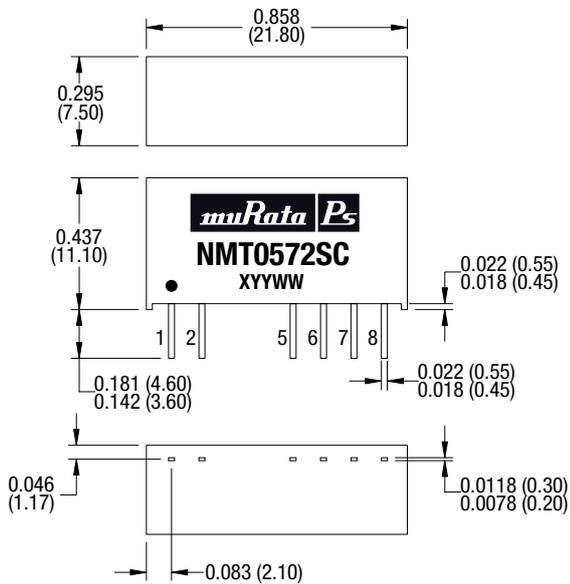
All dimensions in inches  $\pm 0.01$  (mm  $\pm 0.25$ mm). All pins on a 0.1 (2.54) pitch and within  $\pm 0.01$  (0.25) of true position.
