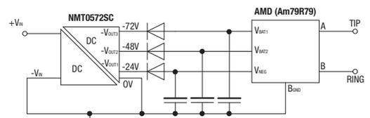
Figure 2. Supply for Ringing SLIC Device
