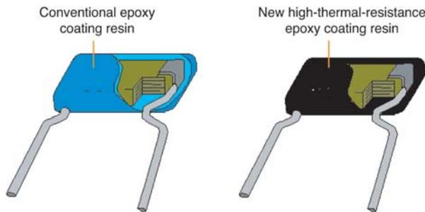
Fig. 1: The internal structure of the lead-type multi-layer ceramic capacitor
