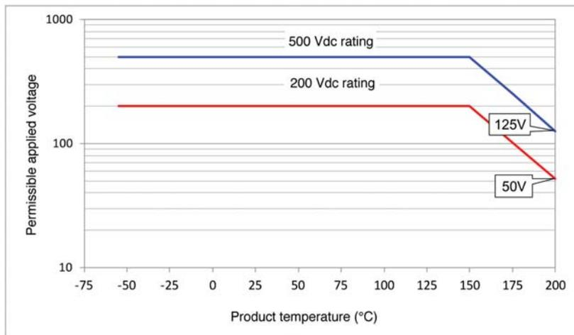
**Fig. 3: Reduction of voltages to be applied**
