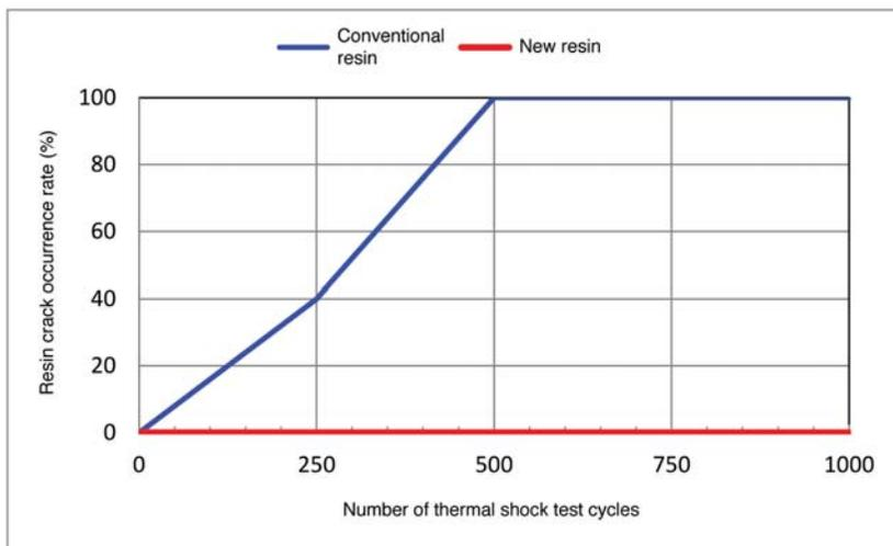
**Fig. 2: Thermal shock test (test conditions: -55°C to +200°C, 1000 cycles)**
