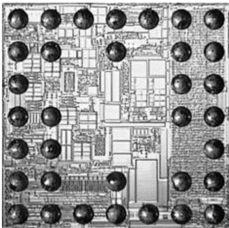
**Figure 1 - Example of a PICS die with the WL-CSP architecture**
