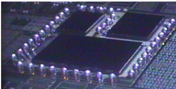
Figure 4 - Sub-system on PICS interposer
