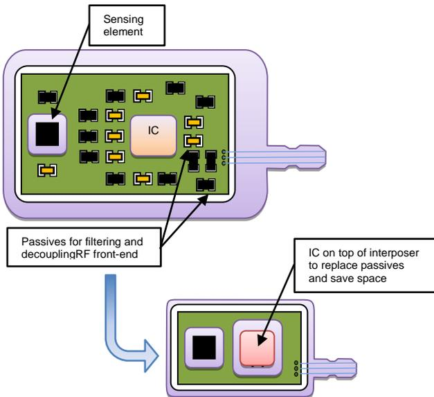
Figure 3 - Architecture evolution with PICS interposer and die stacking
