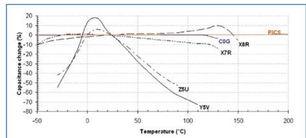
Figure 6 - Temperature performances comparison with various types of MLCC
