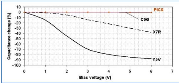
Figure 7 - Voltage stability performances comparisons with various types of MLCC
