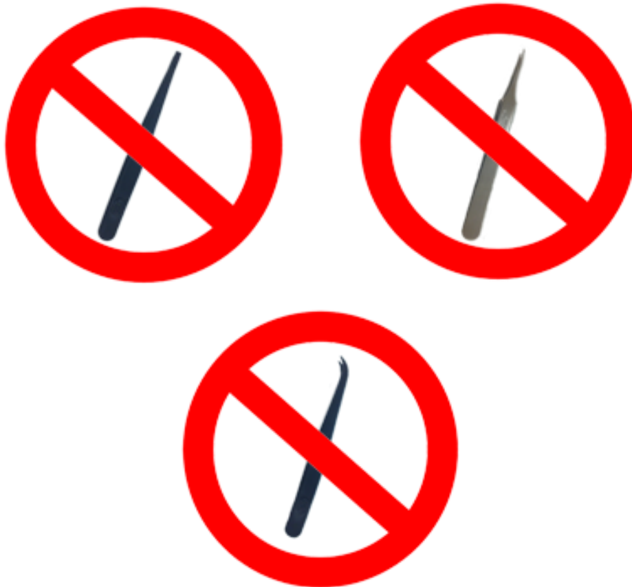
Fig 10. Example of tweezers unsuitable for picking up a die
