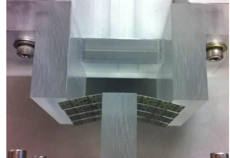
Figure 10: 4PB tool with 4 bent PICS samples
