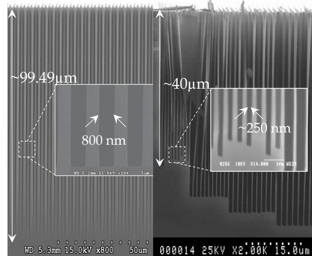
Fig. 1. HAR structures manufactured using the Bosch process: (a) 800nm-wide trenches with a depth of 99.5  $\mu\text{m}$  (aspect ratio 124:1) and (b) 250nm-wide trenches with a depth of 40  $\mu\text{m}$  (aspect ratio 160:1). Some of the walls collapsed during the dicing procedure.
