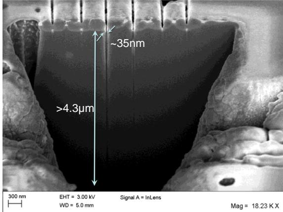
Fig. 2. SEM image of ~35nm trench etched to a depth greater than 4.3 $\mu$ m, hence with aspect ratio >125:1. A rectangular hole was etched using the FIB to allow cross-sectional visualization.
