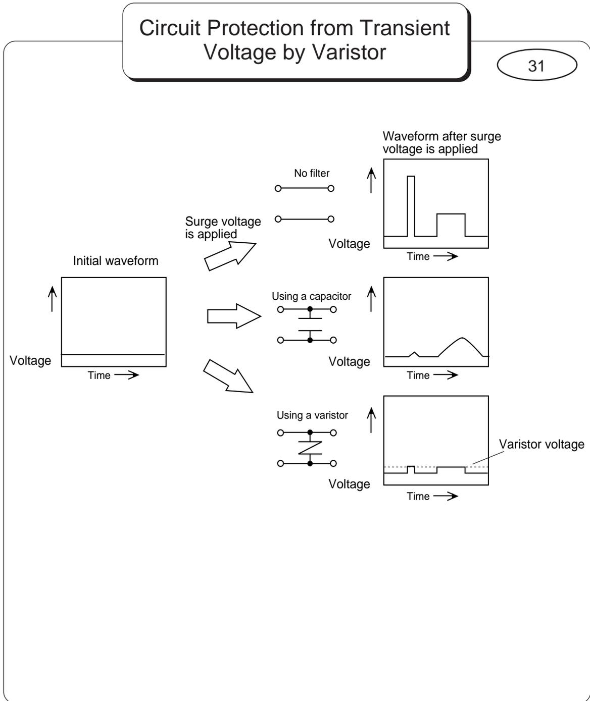
Varistors are used to protect a circuit from high voltage surges.
