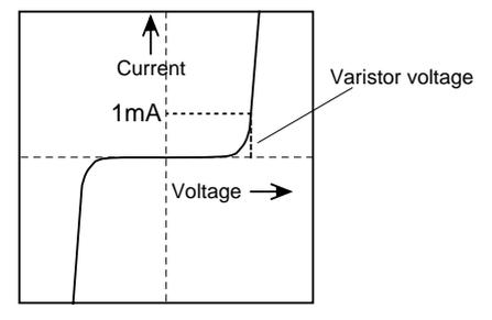
When the surge voltage is equal to or below varistor voltage
