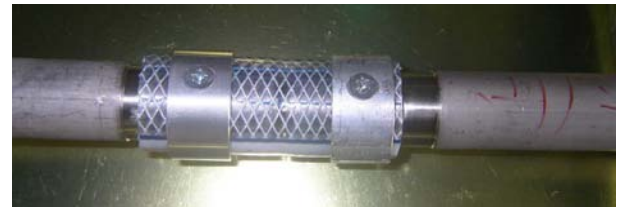
Fig. 10 Flexible connection between pipe segments.
