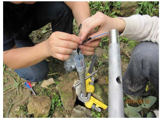
Fig. 11 Waterproof connection between sensor units.
