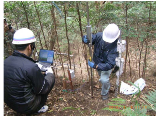
Fig. 4 Installation of miniature ground inclinometer using hammer.
