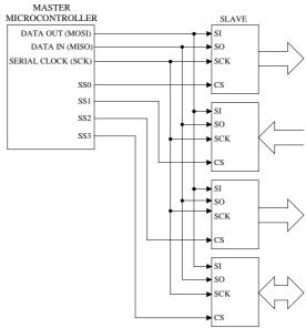
Figure 1. Typical SPI connection
