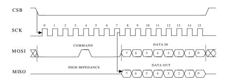
Figure 2. Command and data transmission over the SPI
