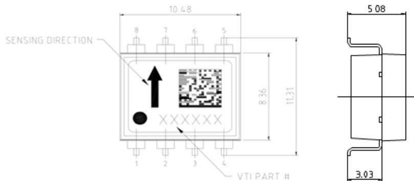
**Figure 8.** Mechanical dimensions (mm).
