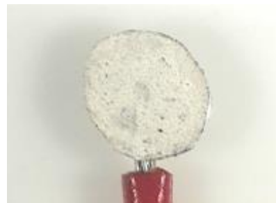
Soldering point where lead wire separation occurred
