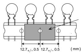
Splicing tape (Base and adhesive tapes are inserted in a splicing tape.
